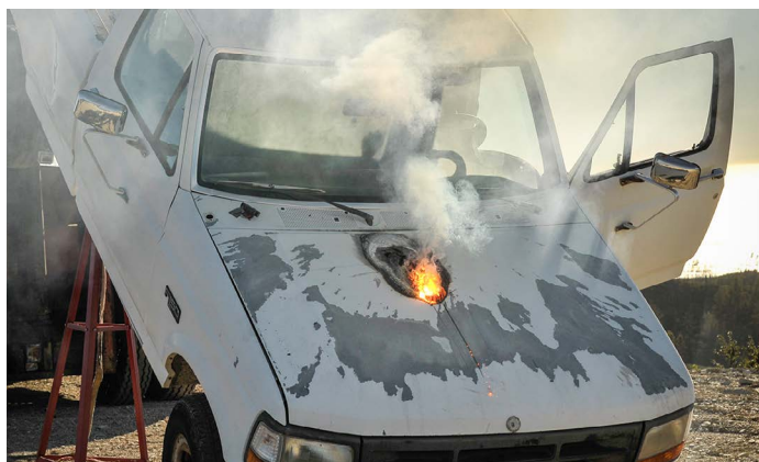
Lockheed Martin ATHENA laser weapon system defeats a truck target by disabling the engine, demonstrating its military effectiveness against enemy ground vehicles. Photo: Lockheed Martin.
