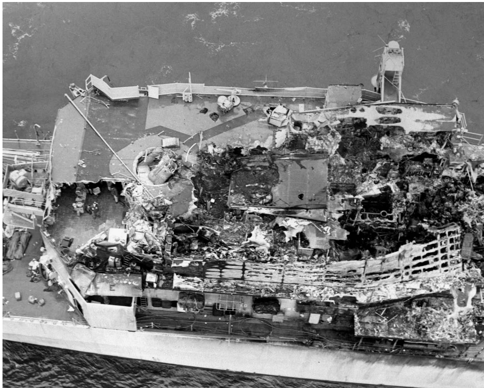
Jet fuel pour down onto USS Belknap when it collided with USS John F. Kennedy. The fuel entered the ventilation system, causing an explosion and fire. U.S. Navy photo)
