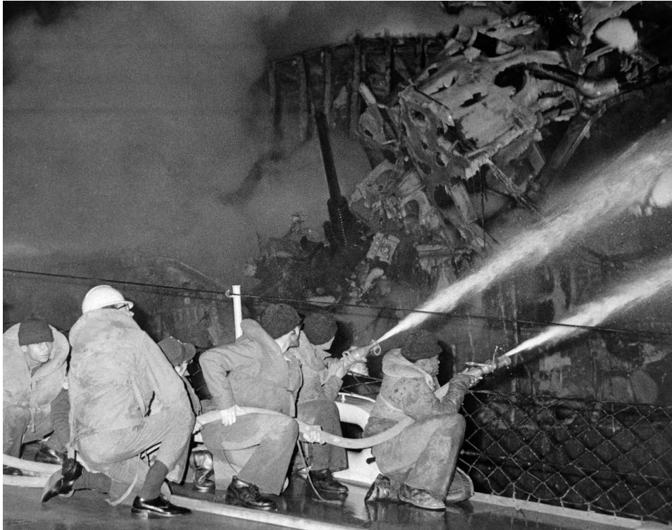
Firefighters aboard the guided missile destroyer USS CLAUDE V. RICKETTS (DDG 5) direct spray from their hoses onto a fire aboard the guided missile cruiser USS BELKNAP (CG 26). The BELKNAP was heavily damaged and caught fire when it collided with the aircraft carrier USS JOHN F. KENNEDY (CV 67) during night operations. (U.S. Navy photo)
